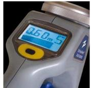
In Sonde/CPS Mode deployed sonde frequencies or Cathodic Protection Systems (CPS) are detected.
