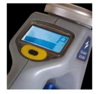
In the P mode the SuperC.AT detects 'power' signals that are being radiated by loaded cables.
