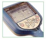
Built for on-site use - IP65 Shock resistant, ingress protected casing protects against
